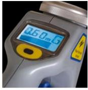
In the G mode the C.A.T<sup>3</sup> detects a tone radiated by the Genny+ to a buried conductor.
