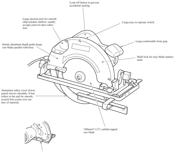
Easy-to-operate lever for adjusting the depth of cut
