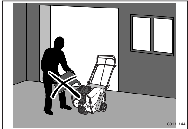
Never fill the fuel tank indoors.
