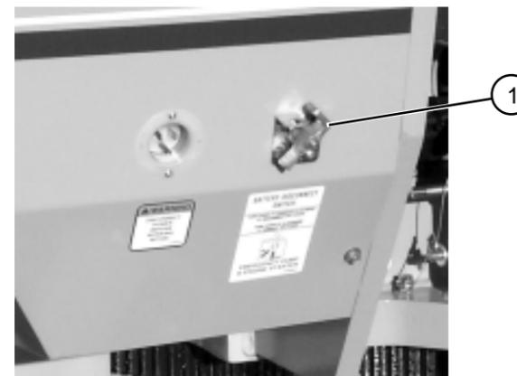
Figure 2-2. Battery Disconnect Switch
