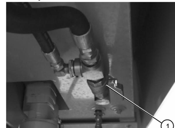
Figure 2-4. Hydraulic Fluid Shut-Off Valve
